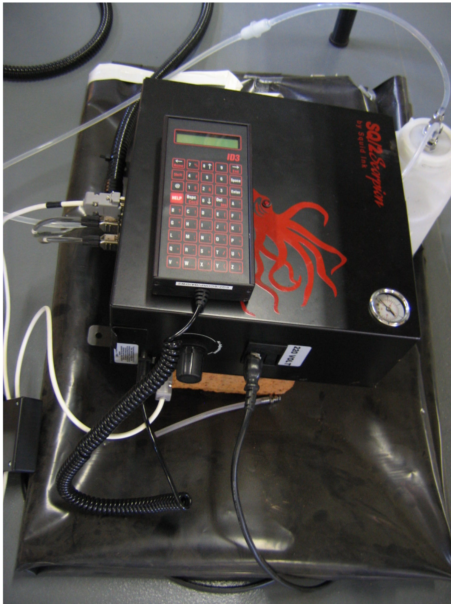
Figure 3.11: Printing system controller unit and ink pressure vessel.
